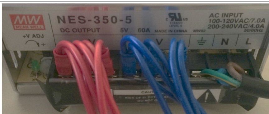
Power supply specifications: Mean Well NES-350-5. DC output 5v 60A. AC input 100-120VAC/7.0A or 200-240VAC/4.0A (the latter for Australia - be sure to correctly set the input switch before using this!) Wiring: Power to the USB hub (ATX connector) from left to right: 3 x Red positive, 3 x Blue negative. Mains power is on the right.
